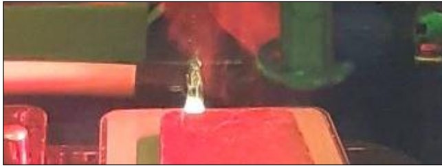
Without Shield gas and extract – poor weld
